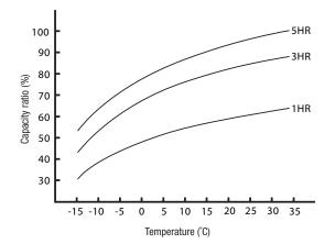
^ Prolonged ambient temperature >35°C for lead acid technologies in material handling applications is a significant factor in reducing the service life of lead acid battery products.
